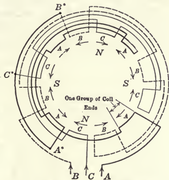
FIG. 27.—General winding diagram for a 3-phase, 4-pole motor with pole-phase groups connected in series star.
